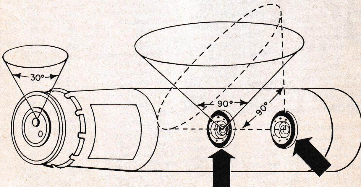
Paths of arming wires from mine to plane should not lead outside the cones drawn here. Heavy arrows point angle of the wire through the safety lock.
