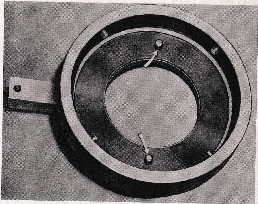
Studs installed in lower half of fixture from Depth-Charge Test Set Mk 2.
