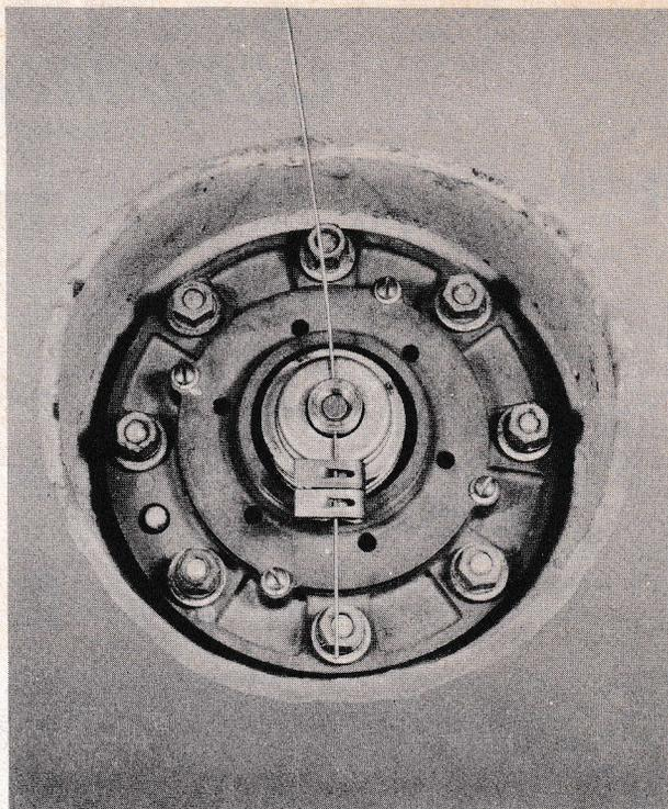
Fahnestock clips must be installed in pairs "upside-down" as shown here. Lashup won't work right when they're installed any other way.
