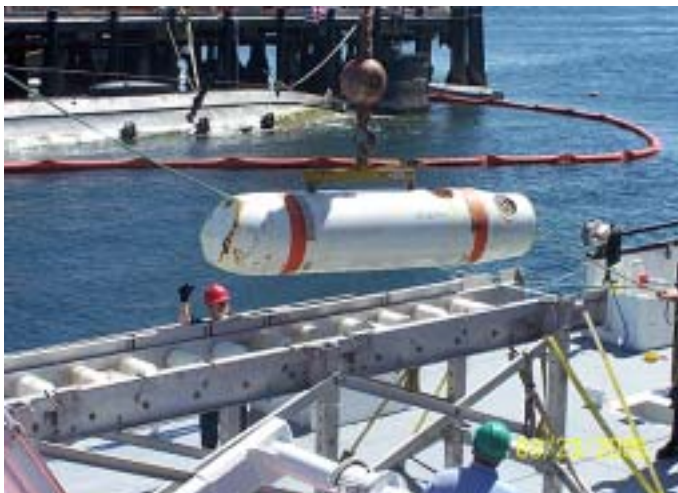
A MK-65, 2,000 lb mine is loaded onto the EX-181 mine rail system to test launching capability on board MV Acoustic Explore in San Diego Harbor. (MN2 Mikael Nissen, MN3 Arlan Madison)
