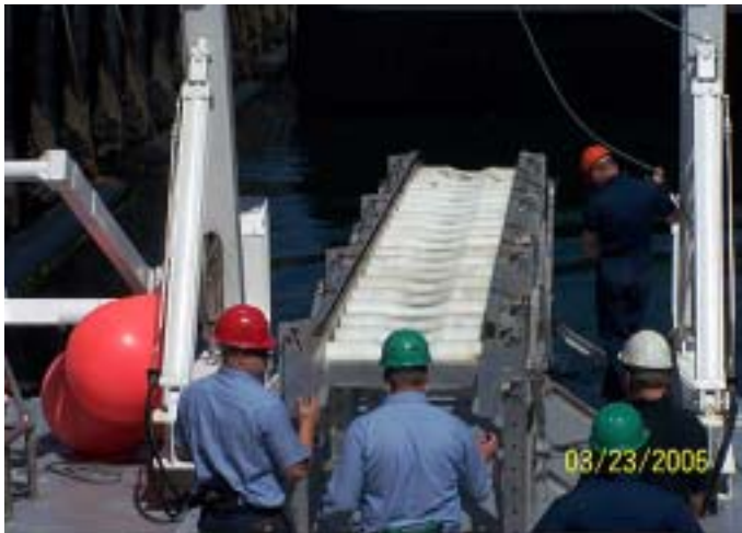
The EX-181 is being aligned for tie down to demonstrate surface mine laying on the MV Acoustic Explore in San Diego Harbor. (MNS Travis Andrews, Master Captain Bob Rosser, MN1 Eddy Gumin, MN3 Arlan Madison, MN3 Brian Danley)
