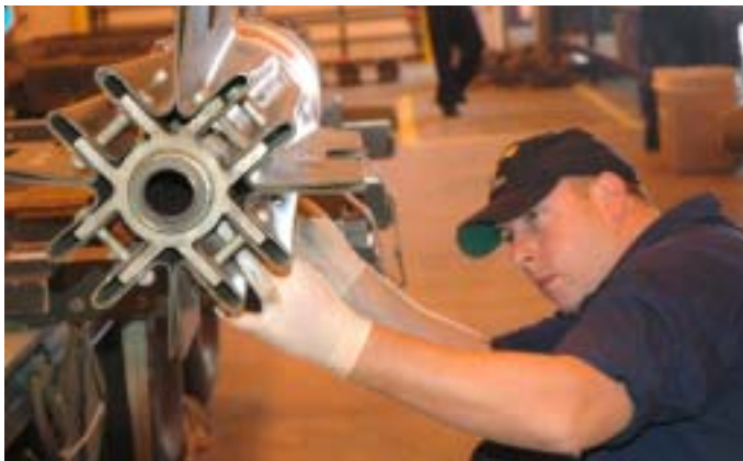
MNSN Petite Inspects MK 9 Arming Wire on Mk 15 Fin
