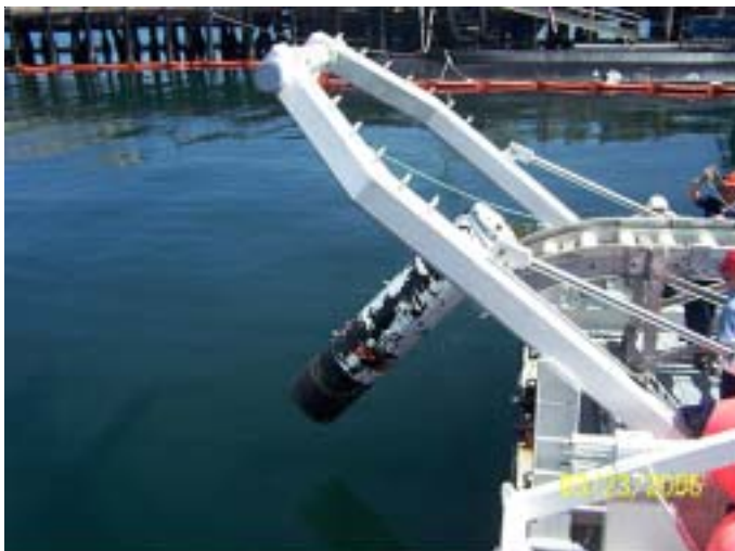
A MK 56, 2,000 lb moored mine is launched form the EX- 181 on board the MV Acoustic Explore in San Diego Harbor. (MN 2 Travis Andrews, MN2 Brian Danley)
