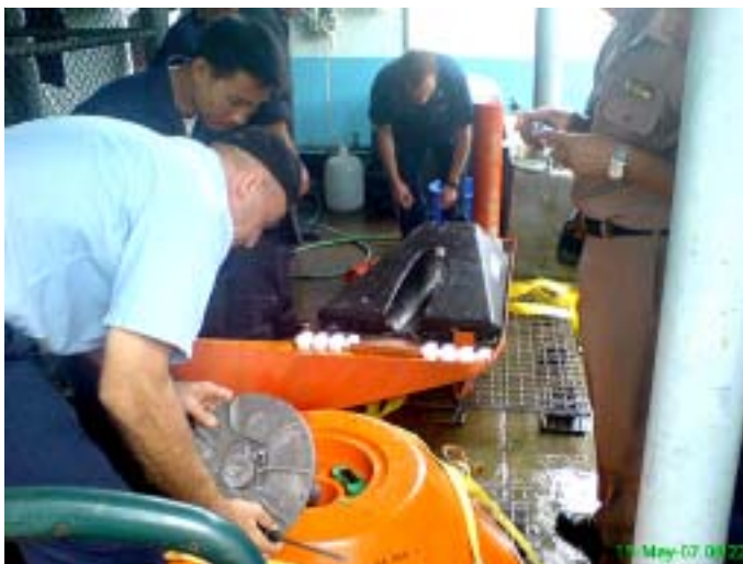
MN1 Quintero and MN3 Shoffner, along with members of the Royal Thai Navy's Mine Prep Shop, perform post-deployment checkout on a MK 44 and MK 46 exercise mine.
