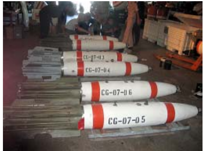
MN1 Quintero and MN3 Shoffner instruct Royal Thai Navy minemen on the assembly and post-inspection of a MK63 Quickstrike mine used during the exercise Cobra Gold '07.
