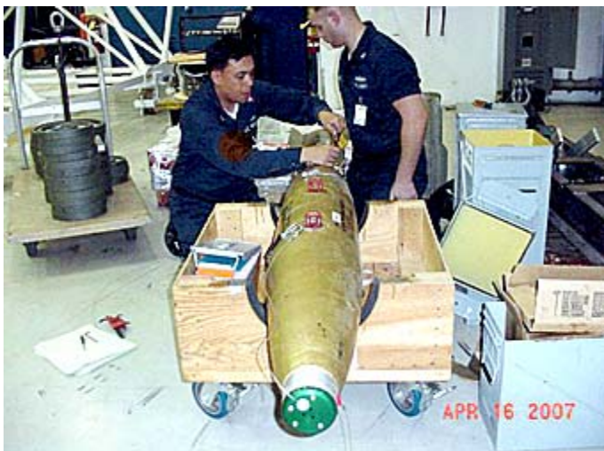
MN1 Walker and MN3 Gardner perform final prep on an MK62 Quickstrike for BRU P-8 testing.
