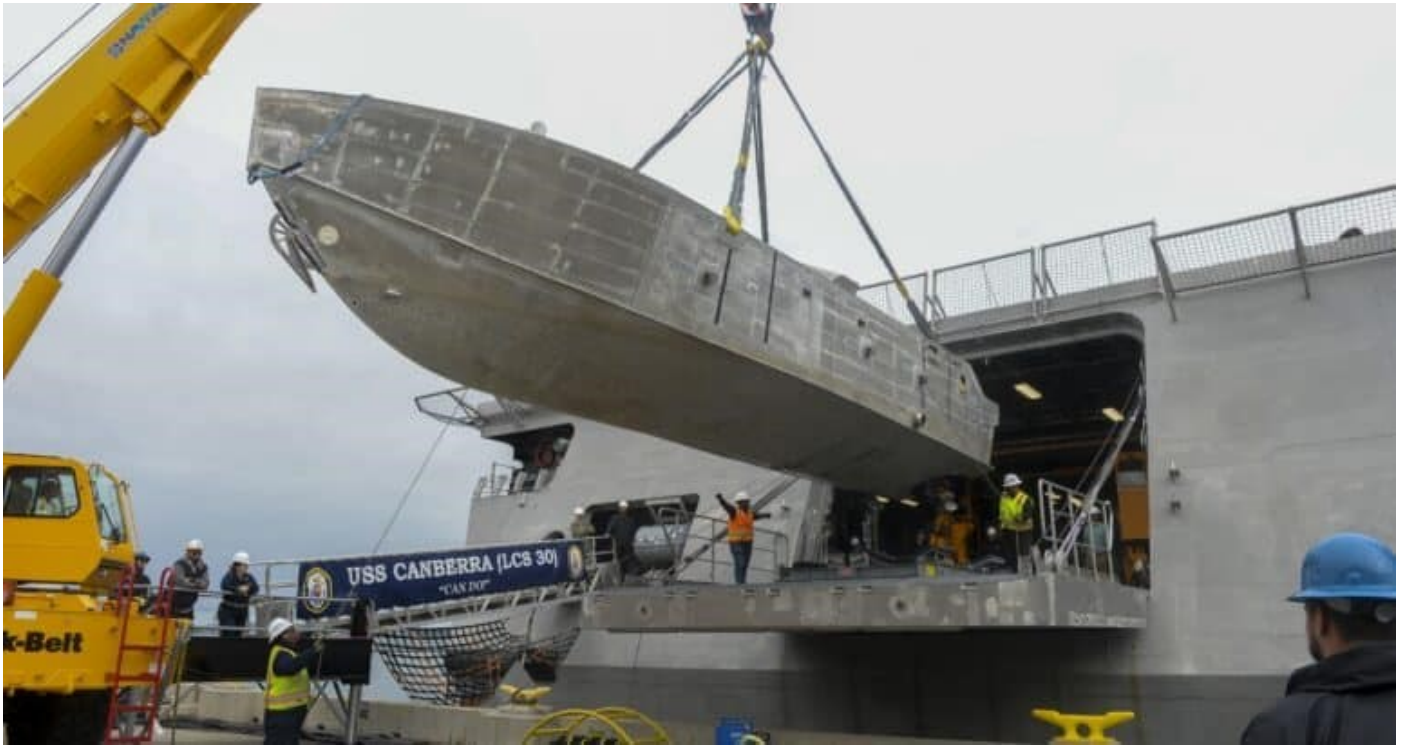
An unmanned surface vehicle is craned aboard the Independence-variant littoral combat ship USS Canberra (LCS 30), as a part of the first embarkation of the Mine Countermeasures (MCM) mission package, April 23. (US Navy photo)
