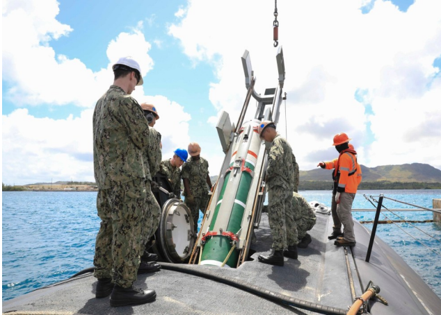
Sailors assigned to the Los Angeles-class fast-attack submarine USS Annapolis (SSN-760) load a MK 67 submarine launched mobile mine (SLMM) onto Annapolis, May 4, 2022. US Navy photo
