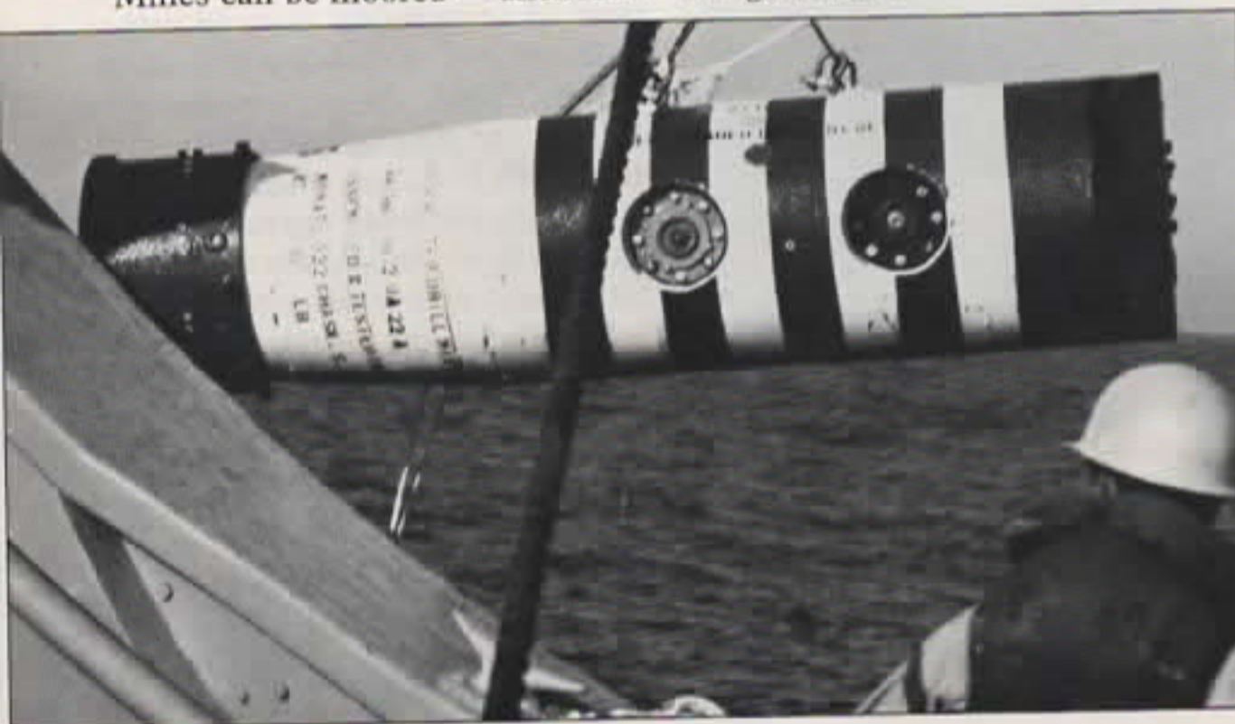
U.S. Navy photo Left: A Mk 36 bottom influence mine is hoisted over the side of a minesweeper during operations off the coast of Charleston, S.C.
