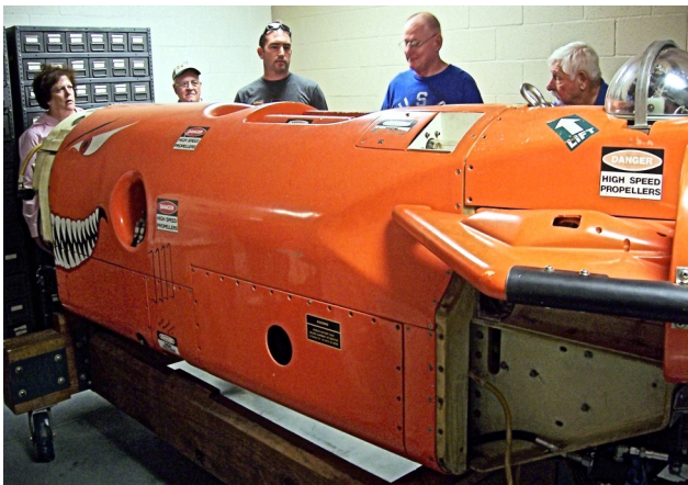
Remote Operated Vehicle (by MN) Cuts Moored Mines, Bomblet for Bottom Mines
