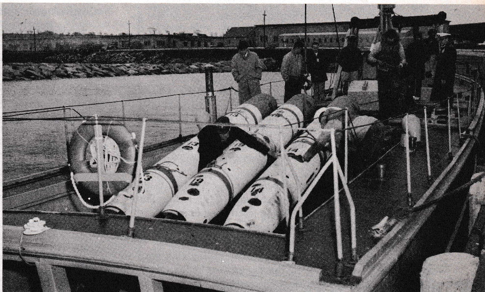
A high speed torpedo retriever is used to gather in the exercise mines at NUOS Gould Island test range. The test site was moved to Newport R.I. because of poor weather on the Chesapeake.
