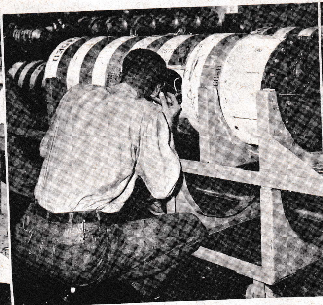
Analysis begins. After checking for case damage and evidence of leaks, O. M. Henry, MN-1 removes and inspects arming device and checks mine fire recorder. Since mine did not fire, recorder should still be running.
