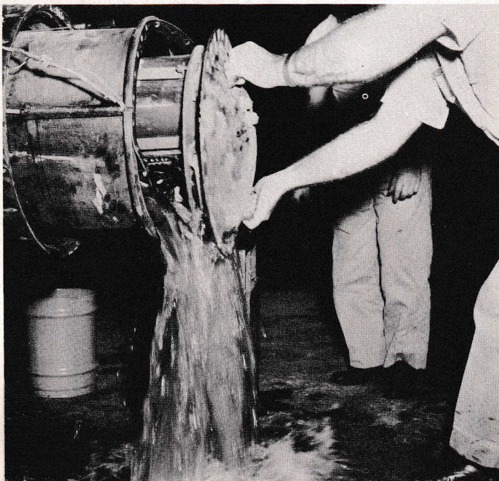
A picture of personnel error. Pressure seals in extension cover weren't tightened.
