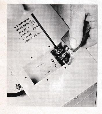
▶ Bunched leads get forced into the battery potting creating a possibility of internal damage.
