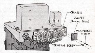
The trouble, we find, is the ground strap that ties terminal 11 of TB-13 to the chassis of the control unit, and thereby to one side of the power source. The remedy is to remove the upper screw from terminal 11, and the mounting screw of the TB-13, and lift off that U-shaped ground jumper. Next, you must put back the terminal 11 screw, not because absence of the ground will interfere with the test, but so the test stand's cable-fanning strip can be attached to the TB-13.
