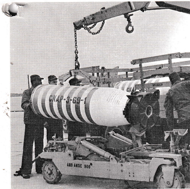
MN3 J.L. Daniel, MNSN D.R. Mick, MN3 T.A. Lawson, and MN1 R.F. Smith (left to right) unload from truck directly onto Aero 33C Bomb Loader . . .
