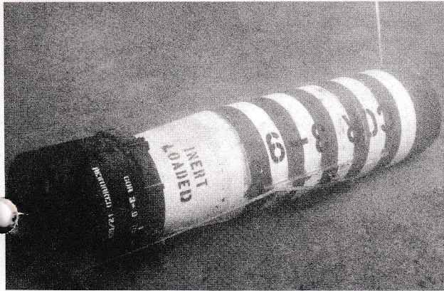
Which goes to prove just how badly fouled a recovery line can get. Apparently the mine rolled over so the line appears to be coming from the wrong end.
