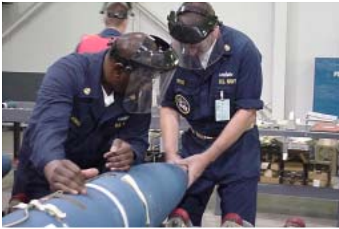
MNC Kent inspecting Arming device installation
