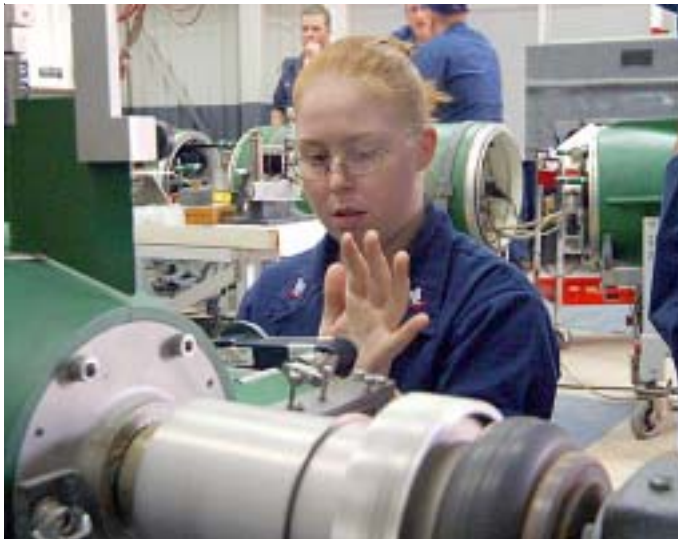
MN3 Sakaris seen here torquing a Surface Control Gage on a SLMM
