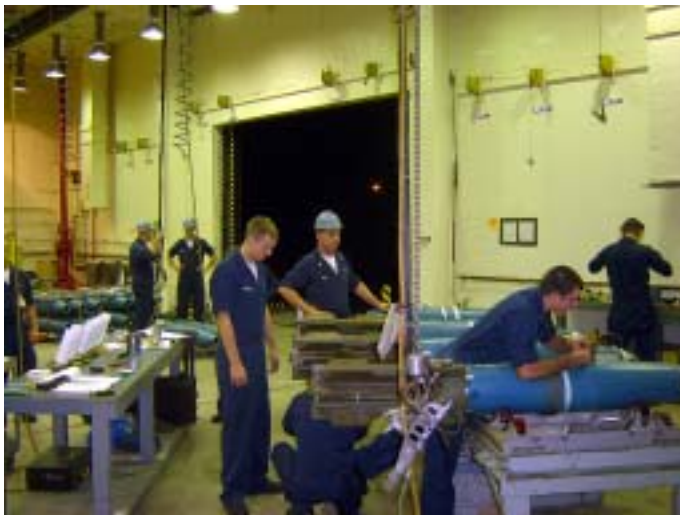
"MOMAU 10 personnel assembling QUICKSTRIKE UMN's MK63 TERMINAL FURY 05"
