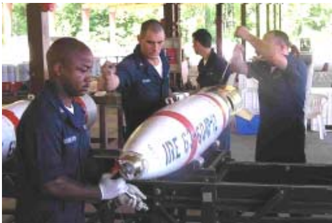
MOMAU 11 personnel assembling MK63 QUICKSTRIKE
